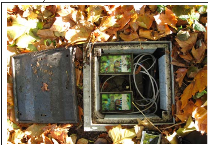
Figure 8 Showing the pedestrian and cyclists counter unit, open and ready for the data to be retrieved.
